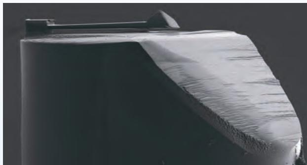
Figure 1: A nano-mechanical sensing device on top of an optical fiber
