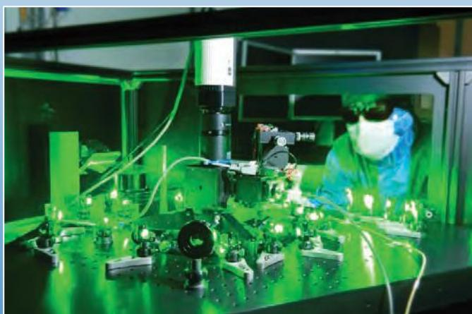
Picture: Rapid nano: Prototype system for high resolution monitoring of particle contamination for the Semicon industry; it is ready to be turned into an industrial product.
