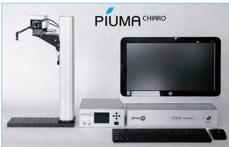
Figure 4: The full Piuma Chiaro system: single cell nanoindentation on an inverted microscope
