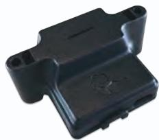
Spark is an ultra-compact sensor that bridges the spectral measurement gap between filter-diode technology and fiber optic array spectrometers. This innovative device provides 5-9 nm resolution from 380-700 nm and is available in standalone and OEM versions, with the level of integration up to the customer.
