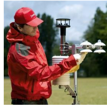
Measurement of net radiation to estimate regional evaporation of water. [Hukseflux Thermal Sensors]
