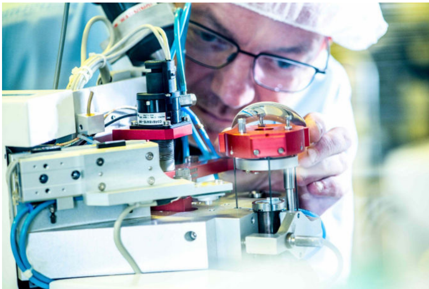
Adjustment of equipment for high volume lens replication (Anteryon)
