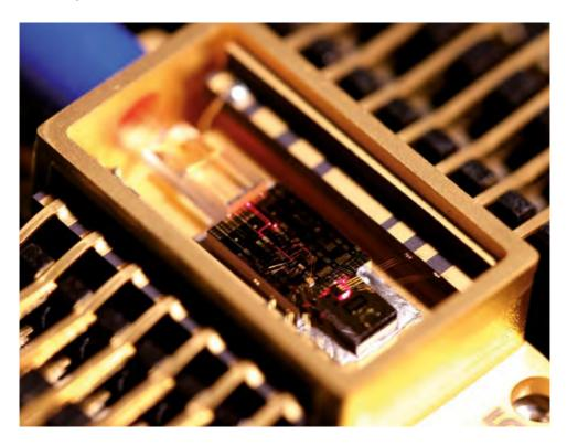
Chilas produces high-end semiconductor external cavity tunable lasers with ultranarrow linewidth,based on hybrid photonic integration technology. Chilas offers wavelength bands around 1550 nm, 850 nm and 780 nm. Chilas lasers are ideal for applications such as; coherent communication, Lidar, fiber sensing, atom cooling, quantum computation and microwave photonics.
